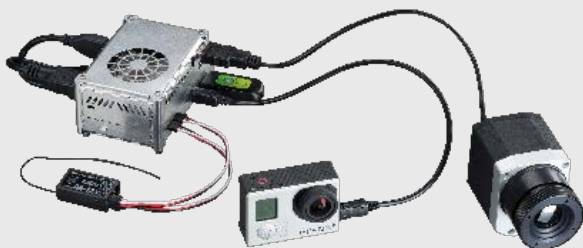
Possible extension with GoPro Hero camera, GPS USB flash drive and 2.4 GHz flight control receiver
